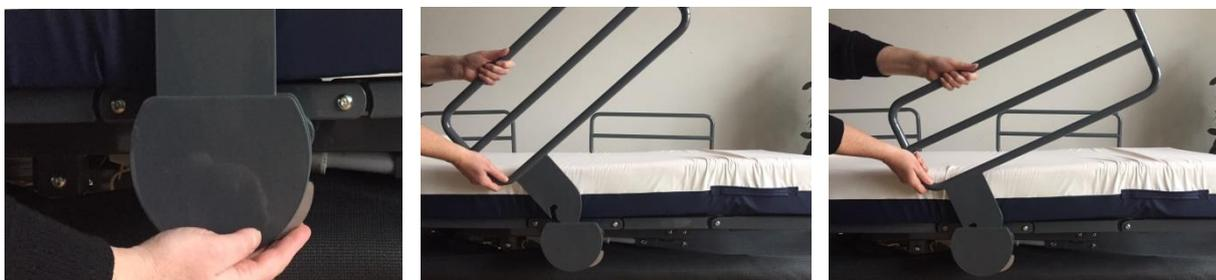
Press the small fitting underneath while lifting the side rail.
